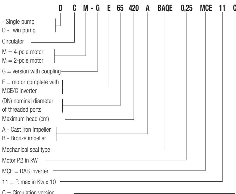
**Installation: horizontal or vertical position, provided that the motor is always above the pump.**
